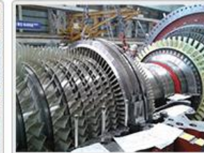
Blade Ring Assembly & Clearance Check
